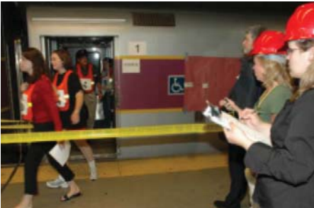
Exiting from Rail Car Egress Experiment Source: fra.dot.gov
