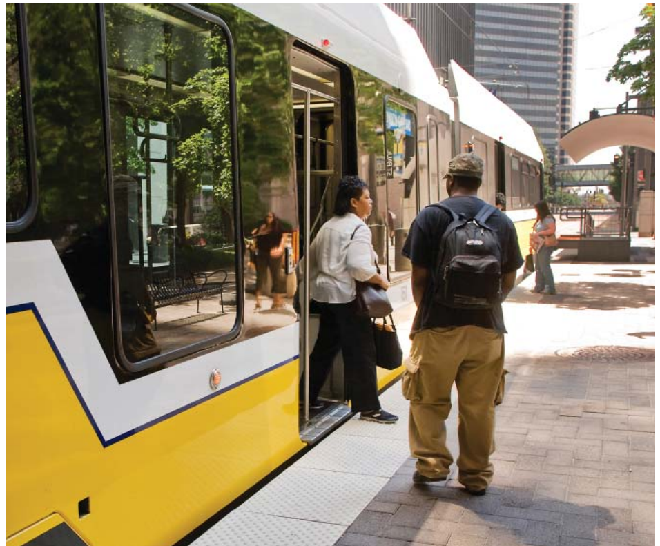
Dallas Area Rapid Transit (DART) St. Paul Station-ADA Compliant Level Boarding source www.dart.org
