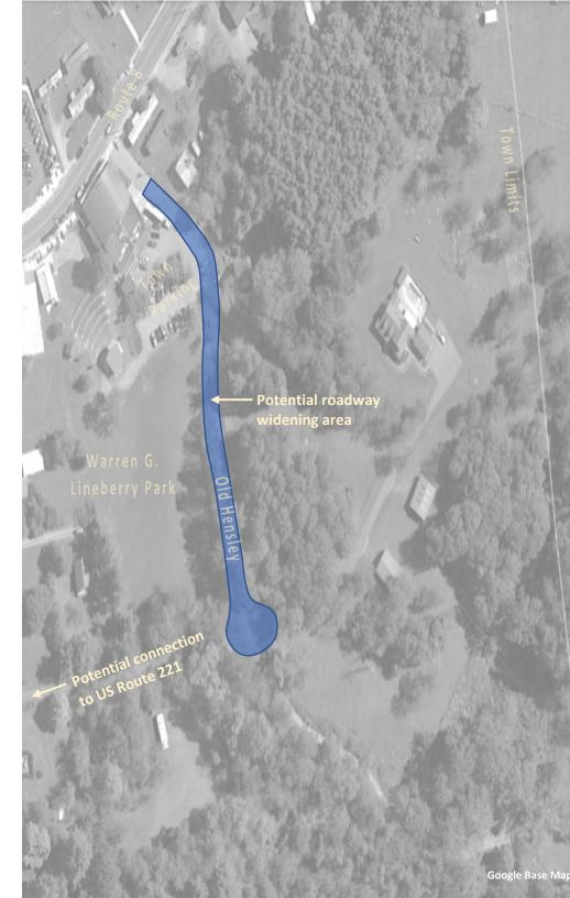
*One-Way Traffic Concept:* Considering the existing right-of-way, which could be limited to a low of 18 feet or a max of 30 feet, converting Old Hensley to a one-way road is another option. To create a one-way route, a connection would need to be created with US Route 221. If the roadway was built to VDOT standards and included a 30-foot right-of-way, the new route could be eligible for state maintenance.
