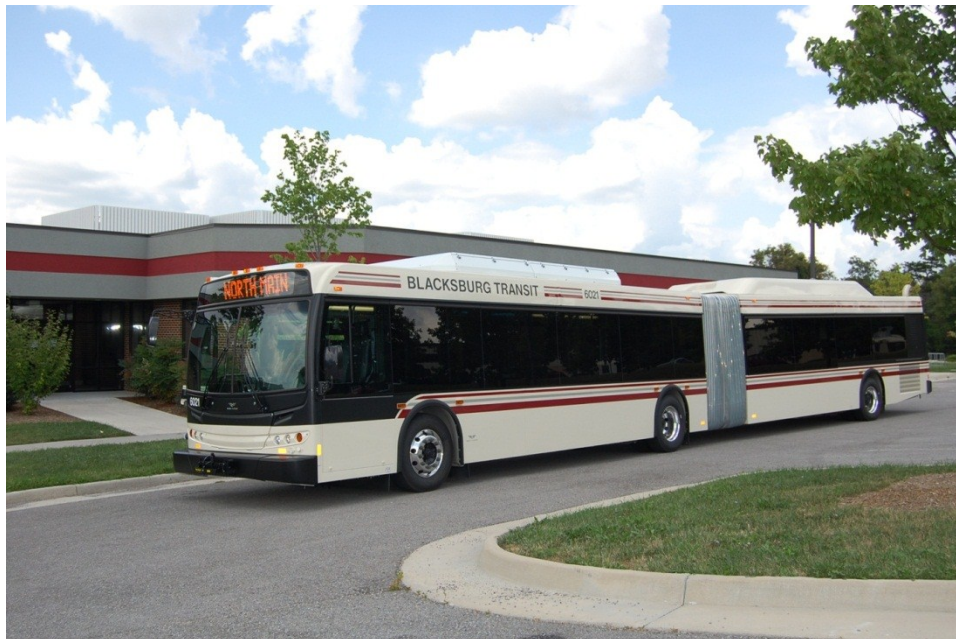
Figure 1-5. BT’s Diesel-Electric Hybrid Articulated Bus
